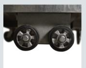
SLOPE Slope system is positioned at the bottom of the brush platform. Slope angle is adjustable over command button.
